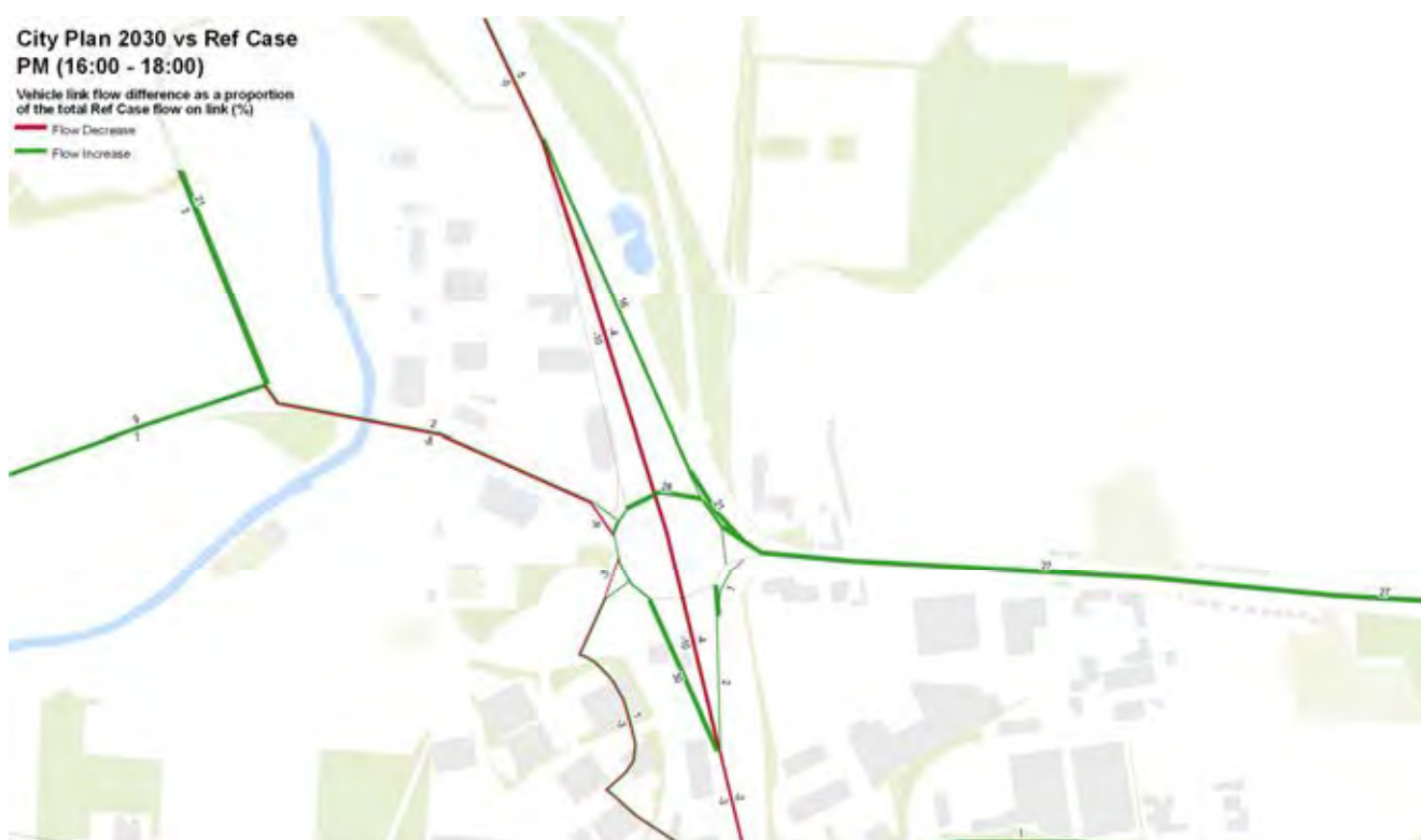
Figure 2.4: PM City Plan (Brownfield with IBG2) vs Ref Case – proportional (%) difference in flow relative to total Ref Case link flow
