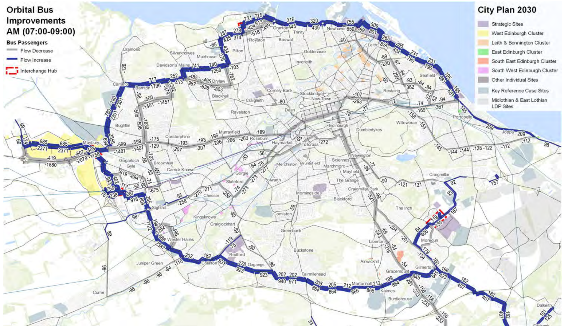
Figure 6.17: Public Transport model flow changes following introduction of improved orbital bus services
