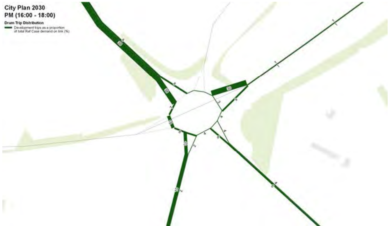
Figure 3.18: PM distribution of Drum only trips relative to Ref Case link demand
