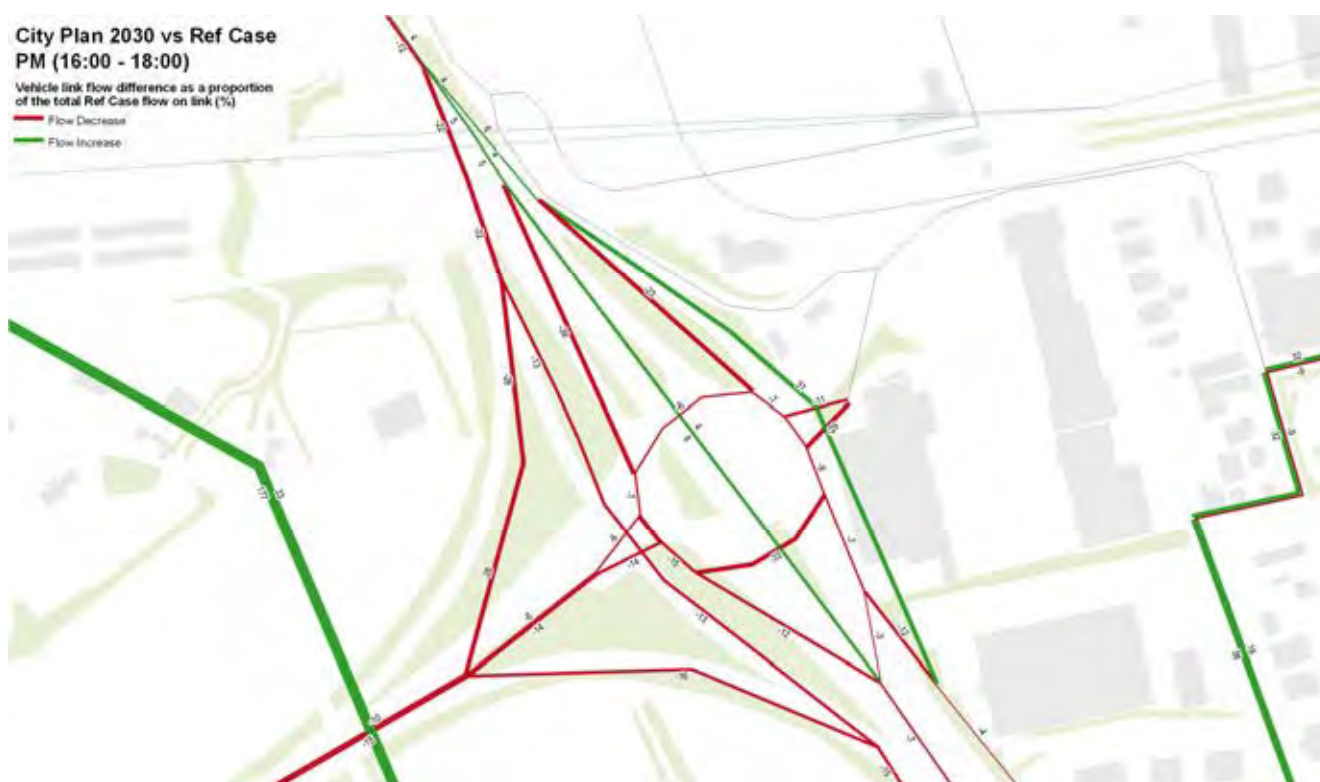
Figure 3.10: PM City Plan (Brownfield with Drum) vs Ref Case – proportional (%) difference in flow relative to total Ref Case link flow
