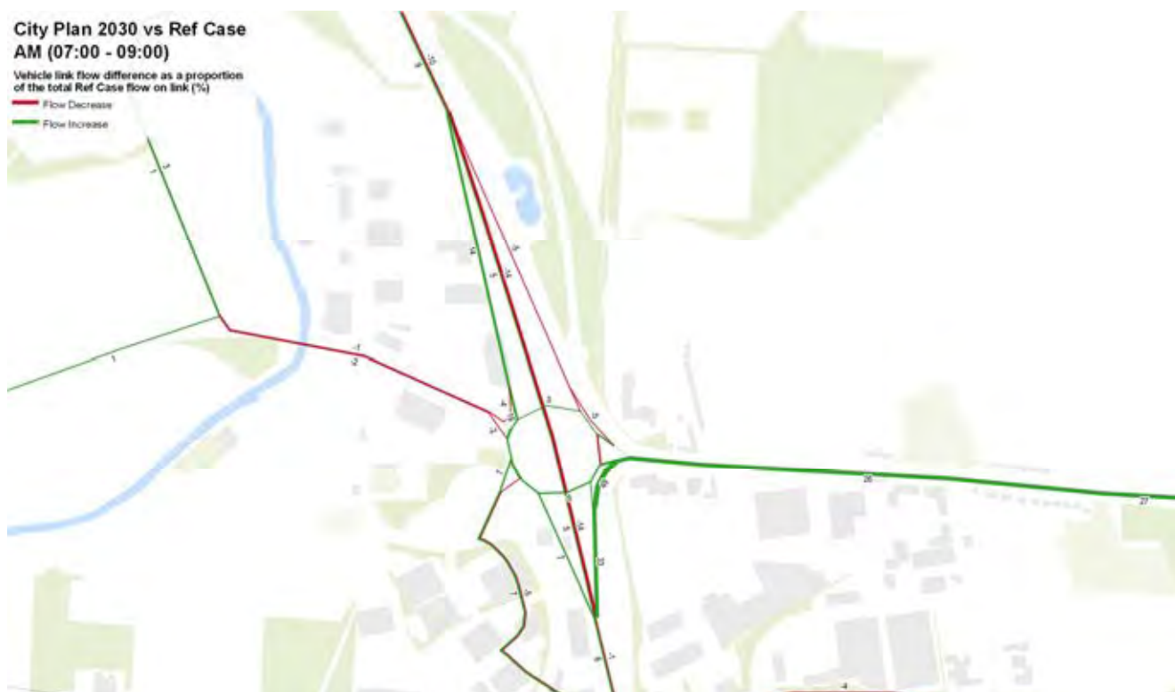
Figure 3.1: AM City Plan (Brownfield with Drum) vs Ref Case – proportional (%) difference in flow relative to total Ref Case link flow
