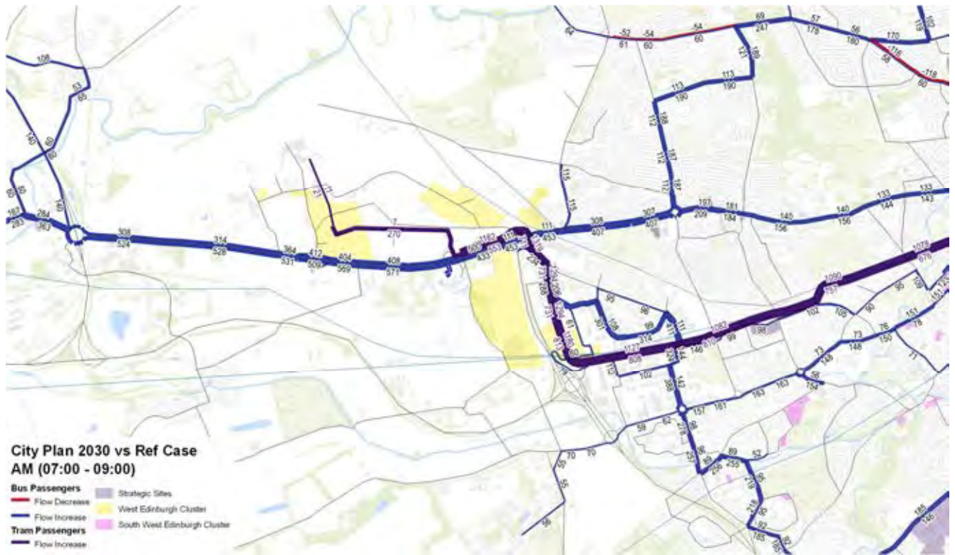
Figure 5.12: City Plan 2030 Brownfield with Drum vs Reference Case Public Transport Model Flow Difference Plot – West Edinburgh
