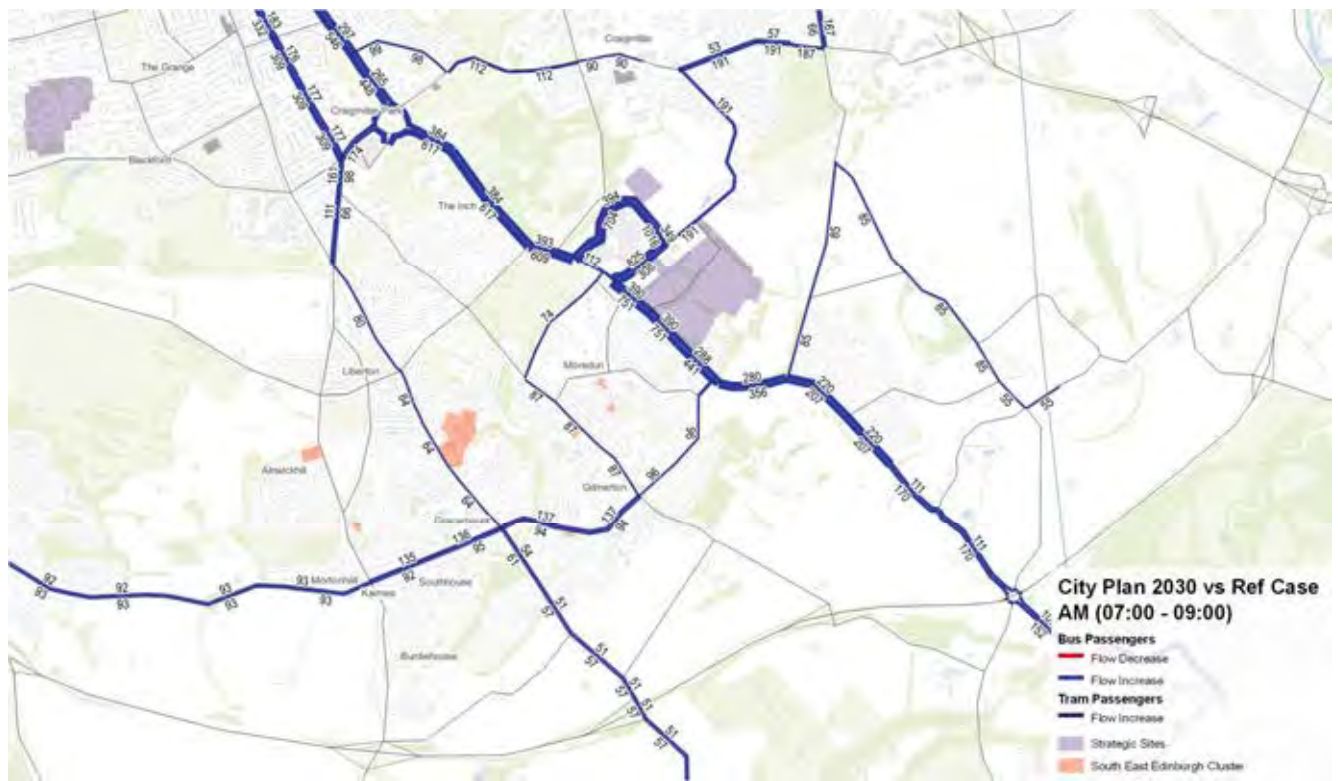
Figure 5.8: City Plan 2030 Brownfield with IBG2 vs Reference Case Public Transport Model Flow Difference Plot – South East Edinburgh
