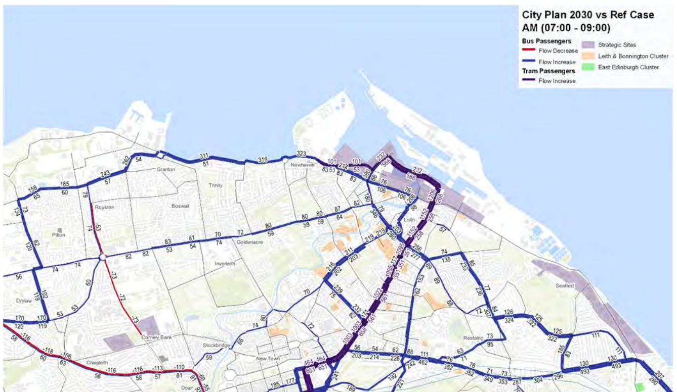
Figure 5.19: City Plan 2030 Brownfield with IBG2 vs Reference Case Public Transport Model Flow Difference Plot – North Edinburgh
